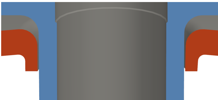
Figure 4: The annular gap is the orifice formed by the pintle outer diameter and the injector face
